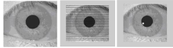
Fig Detecting the rectangular area. (a) Iris image, (b) The lines that were drawn to detect rectangular areas, (c) The result of detecting of rectangular area
