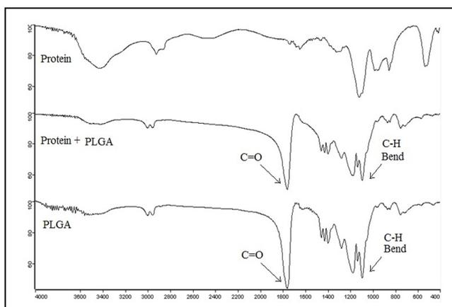
Figure 3. The FTIR spectra of AAT, PLGA+ AAT and PLGA NPs.
