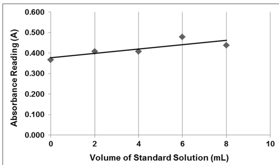
Figure 3. Linear Regression of the absorbance readings (y-value) against the volume of arginine standard solution in mL (x-value) for Sample 3
