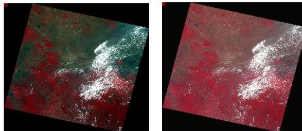
Fig. 4 Comparison of 2009 image before and after FLAASH (left: before; right: after)
