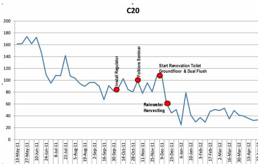
Fig 4: Meter readings for C20 (Main Building)
