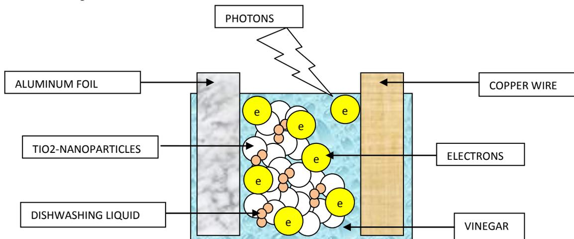
Fig. 1: Simulated Characteristics of TiO<sub>2</sub>-Based Sensitized Solar Cell Using Vinegar
