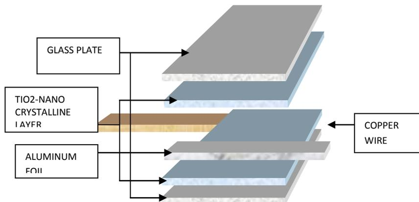
Fig. 12: Configuration of TiO<sub>2</sub>-Based Sensitized Solar Cell Using Vinegar
