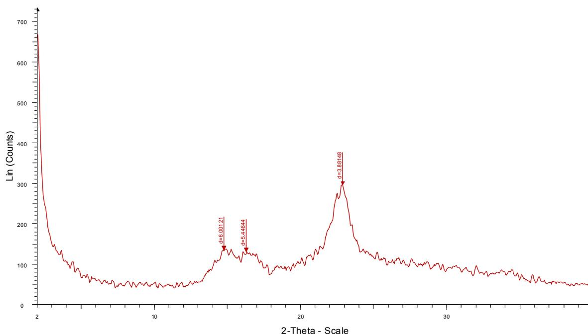
Fig. 1: X-Ray diagram for obtained nano crystalline cellulose
