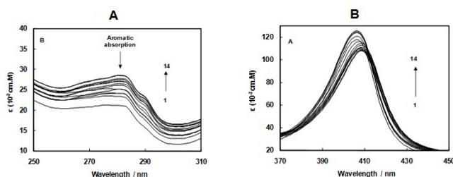
Fig. 4: Effect of urea on (A) surar absorption line, and (B) aromatic absorption 30 μM cytochrome c in 100 mM phosphate buffer, the concentration of urea, respectively 0, 1, 2, 3, 4, 5, 5.5, 6, 6.5, 7, 7.5, 8, 8.5, 9 and 9.5 M.
