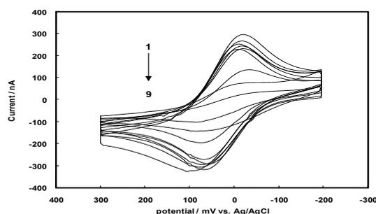
Fig. 1: Voltammogram cycle of cytochrome c. Voltammogram were obtained to the concentrations of 0, 1, 2, 3, 4, 5, 6, 7 and 8 M urea, orderly. 20 mM phosphate buffer and 100 mV/s probe speed.
