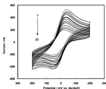
Fig. 6: Effect of different concentrations of SDS on the electrochemical response of cytochrome c; respectively, from top to bottom: 0.1, 0.2, 0.3, 0.4, 0.5, 0.6, 0.7, 0.8, 0.9, 1, 2, 3, 4, 5, 6, 7, 8, 9, 10, 12, 14, 16, 18, 20, 22, 24 and 26 mM. Protein concentration of 100 mM, gold electrode modified with 2-mercaptoethanol, 20 mM of buffer.
