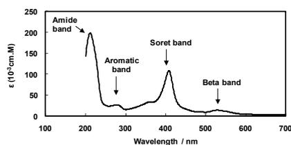
Fig. 3: Absorption spectrum of Uv-Vis of 30 μM cytochrome c in 100 mM phosphate buffer.
