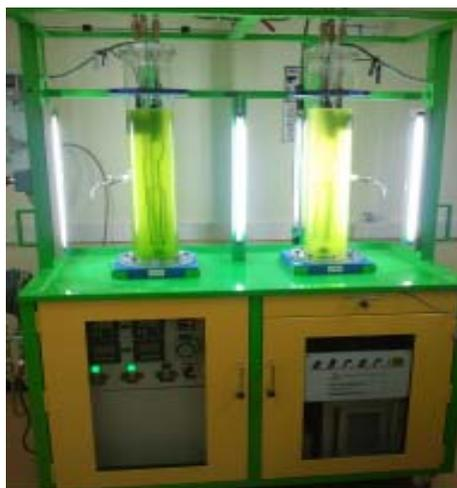
Fig. 1: A 2x10L photobioreactor used in the experiment
