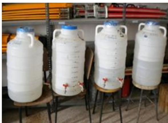
Fig. 2: A sample plastic tanks having different salt concentrations
