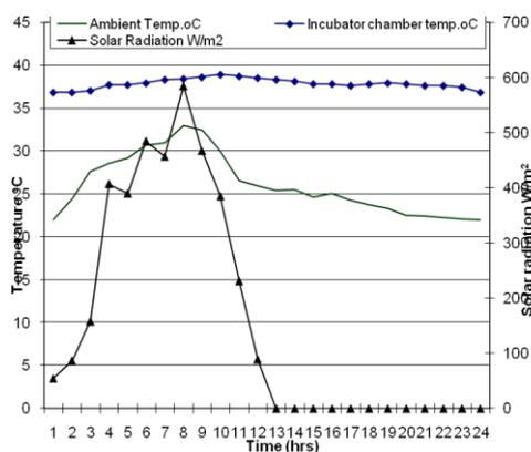
Fig. 4: Ambient and incubator temperature profiles with time.
