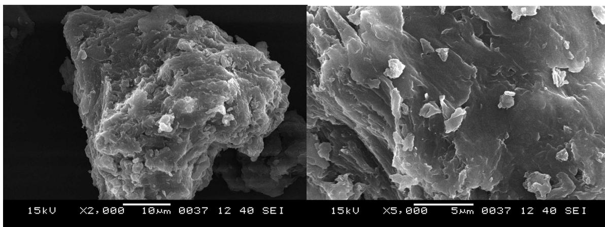
Fig. 2: Scanning Electron microscope image of cobalt ferrite nanoparticles
