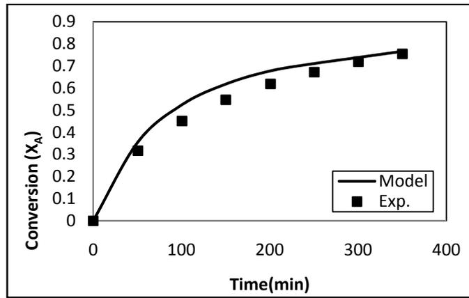
Fig. 6: Comparison of experimental and model results for acetic acid conversion ( $M = 1.5$ ,  $T = 70^{\circ}\text{C}$ )
