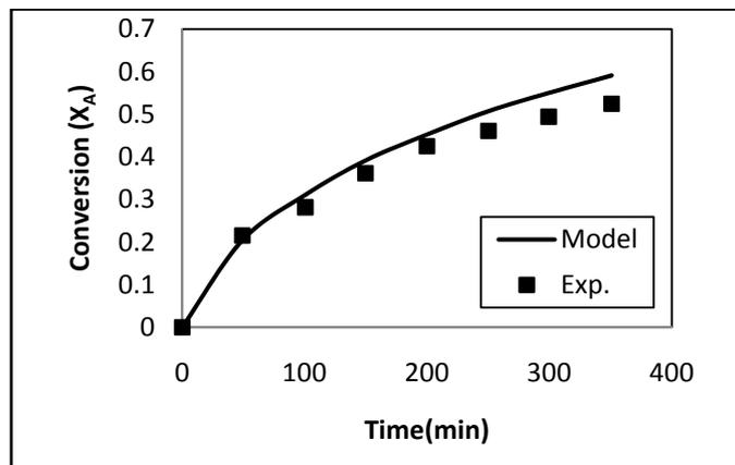
Fig. 4: Comparison of experimental and model results for acetic acid conversion ( $M = 1.5$ ,  $T = 50^\circ\text{C}$ )
