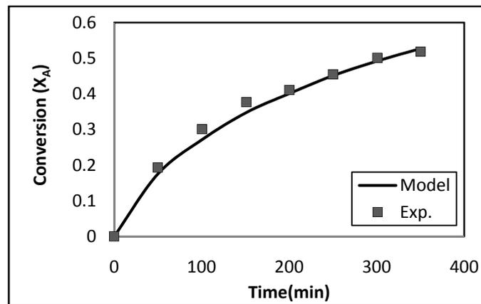
Fig. 1: Comparison of experimental and model results for acetic acid conversion (M = 1, T = 50°C)
