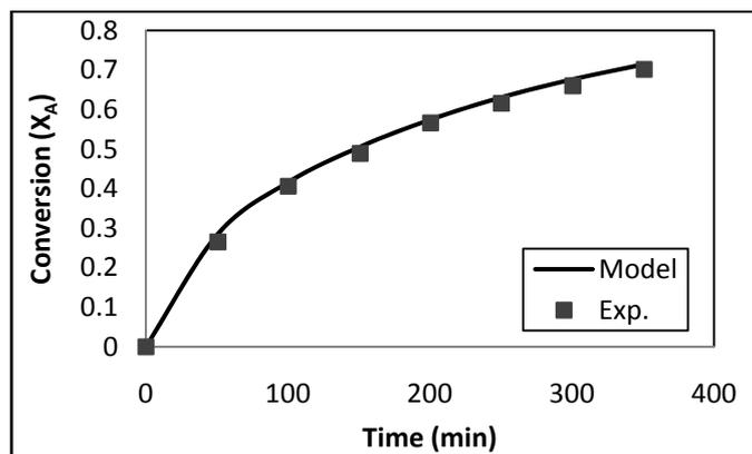
Fig. 5: Comparison of experimental and model results for acetic acid conversion ( $M = 1.5$ ,  $T = 60^\circ\text{C}$ )
