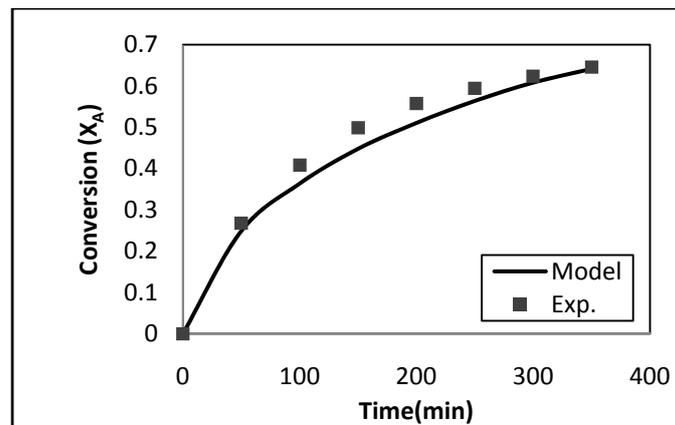
Fig. 2: Comparison of experimental and model results for acetic acid conversion (M = 1, T = 60°C)
