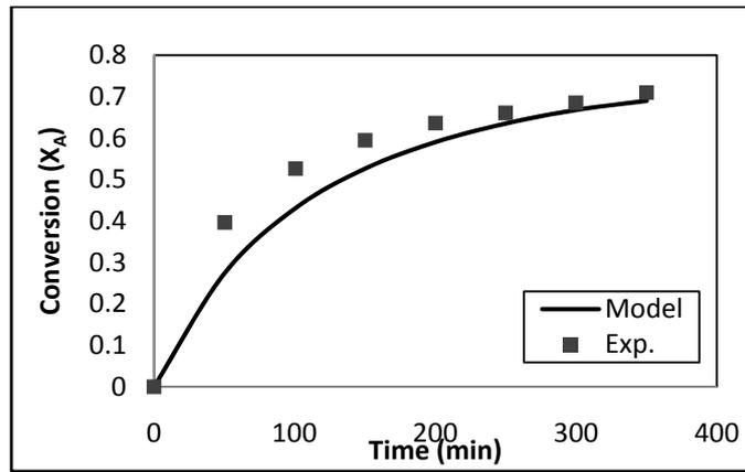
Fig. 3: Comparison of experimental and model results for acetic acid conversion ( $M = 1$ ,  $T = 70^\circ\text{C}$ )
