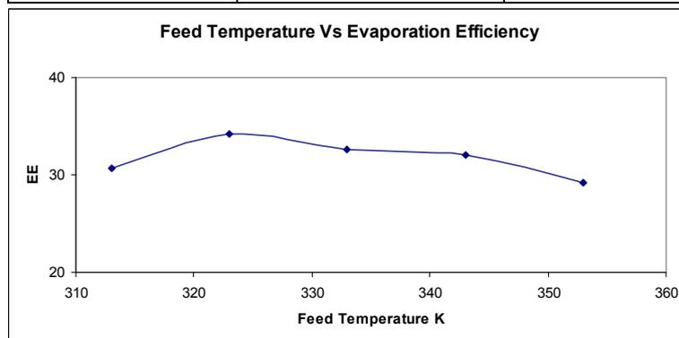
Fig. 1: Effect of feed temperature on Evaporation Efficiency.
