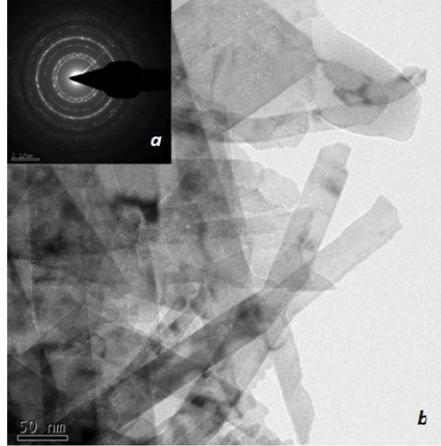
Fig. 2: (a): Select-area electron diffraction (SAED) of as prepared CuO nanoparticles (b): Typical TEM micrograph for synthesized rod shaped nanoparticles
