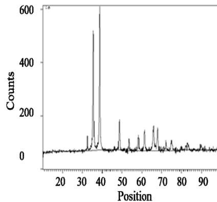
Fig. 1: XRD graph for CuO nanoparticles prepared with single step chemical synthesis method.
