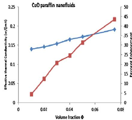
Fig. 3: CuO paraffin nanofluids effective thermal conductivity and percent enhancement in thermal conductivity
