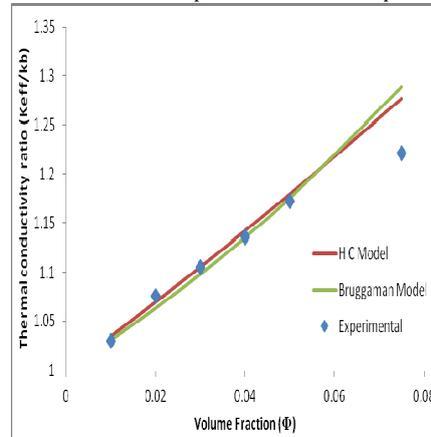
Fig. 4: Comparison of ratio of experimental thermal conductivity ratio and model-predicted ratio.
