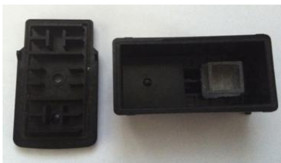
Fig. 3: The modified ink cartridge
