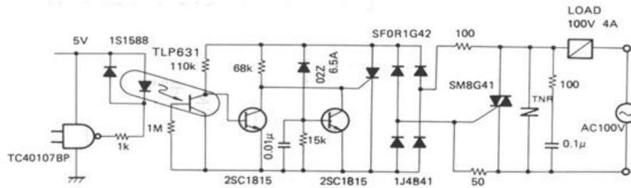
Fig. 2: A schematic diagram of zero crossing SSR.
