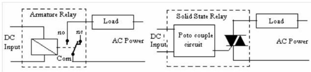
Fig. 1: A schematic diagram of the two relays.
