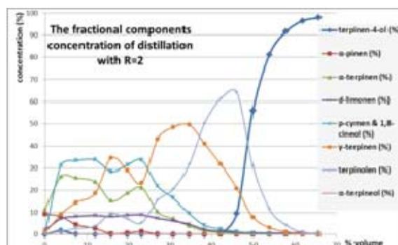
Fig. 6: The fractional components concentration of distillation with R=2.
