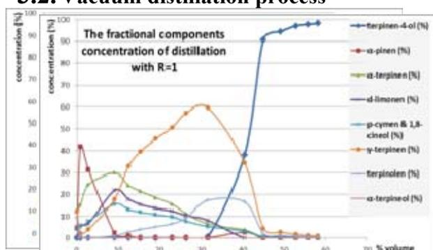
Fig. 5: The fractional components concentration of distillation with R=1.
