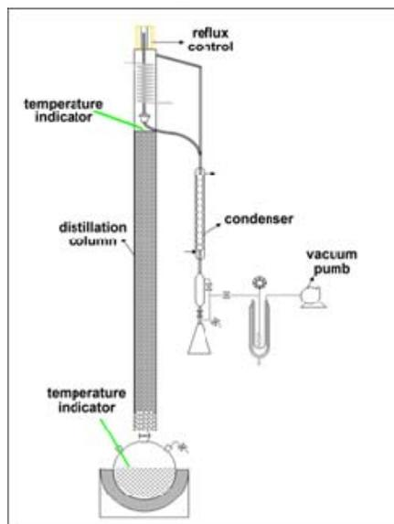
Fig. 2: The vacuum distillation system
