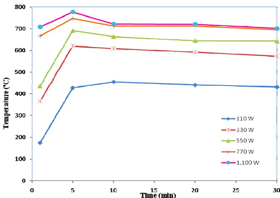
Fig. 2: The temperature profiles under different microwave power
