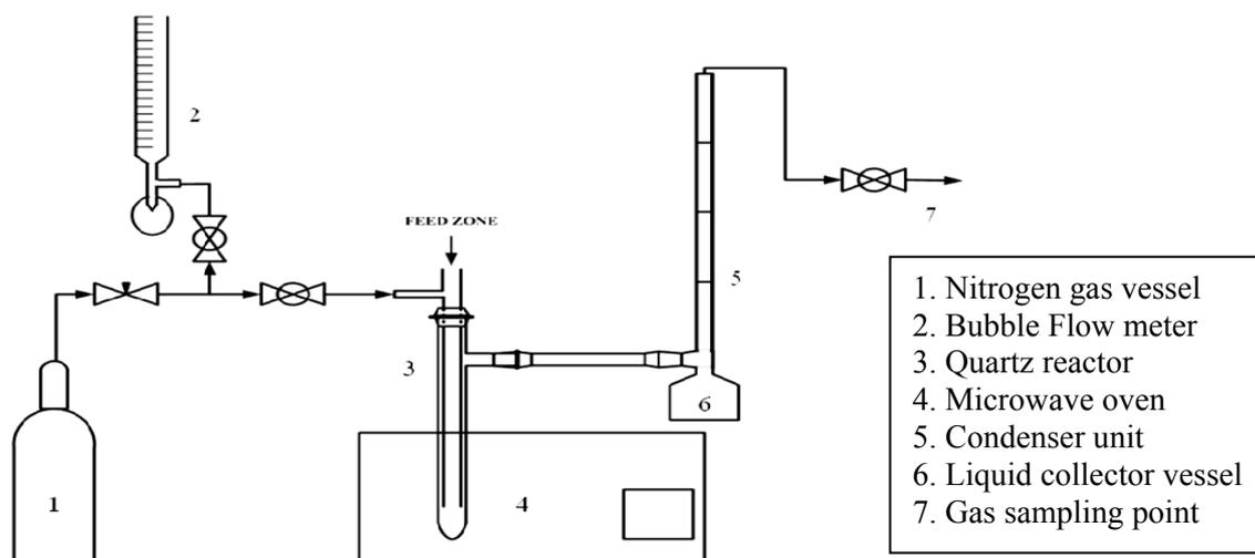
Fig. 1: Schematic layout of microwave pyrolysis system.
