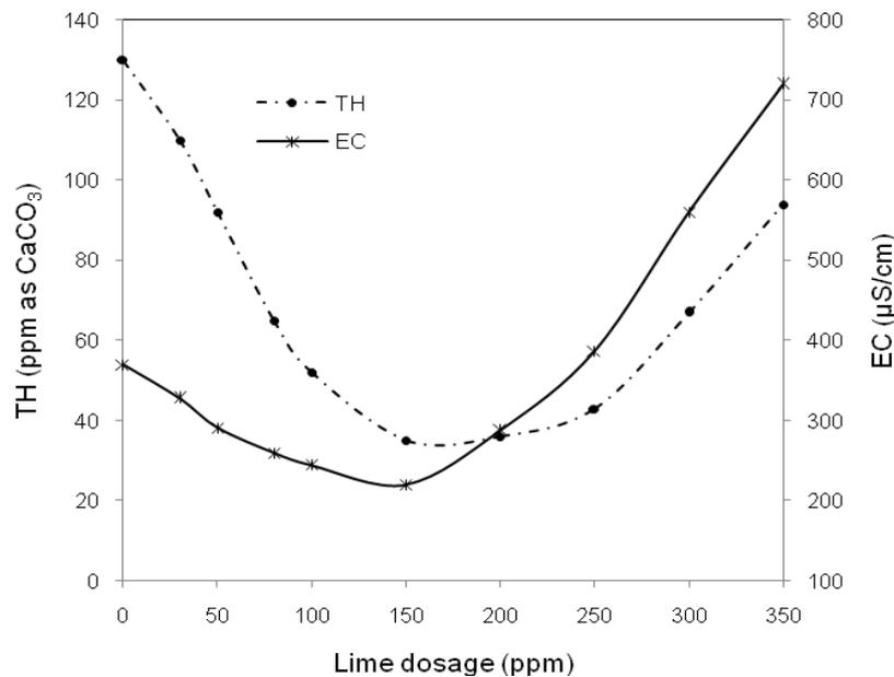
Fig. 2: Changes of TH and EC versus lime dosage at ESC clarifier feed water
