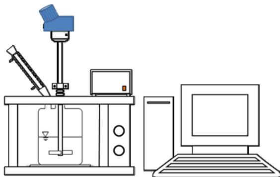
Fig. 1: Schematic diagram of modified domestic microwave oven for batch experiments.
