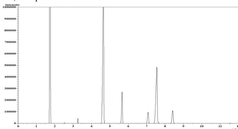
Fig. 2: GC chromatogram of palm stearin biodiesel at 50 s of irradiation time, 7:1 methanol to oil molar ratio, 60 °C, 0.5% NaOH, 600 rpm of mixing speed and 0.15 W/g of palm stearin.
