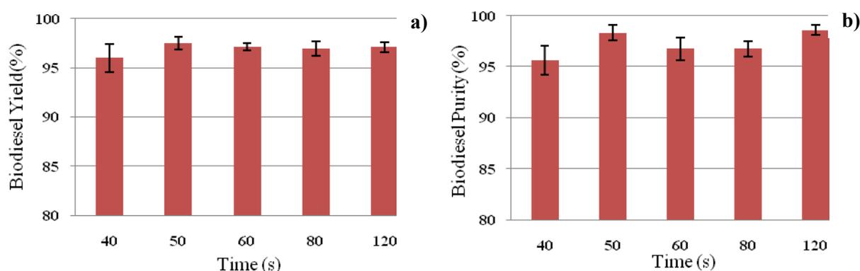
Fig. 3: Effect of radiation times on a) biodiesel yield, b) biodiesel purity at 7:1 methanol to oil molar ratio, 60 °C, 0.5% NaOH, 600 rpm of mixing speed and 0.15 W/g of palm stearin.
