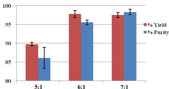
Fig. 4: Effect of methanol to oil molar ratios on biodiesel yield and purity at 50 s of radiation time, 60 °C, 0.5% NaOH, 600 rpm of mixing speed and 0.15 W/g of palm stearin.
