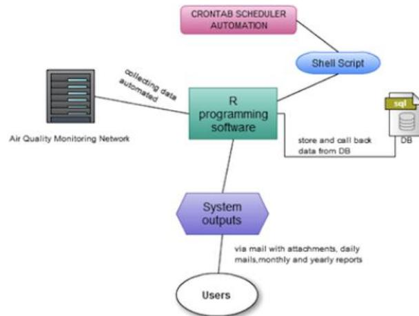
Fig. 2. 1: System Architecture
