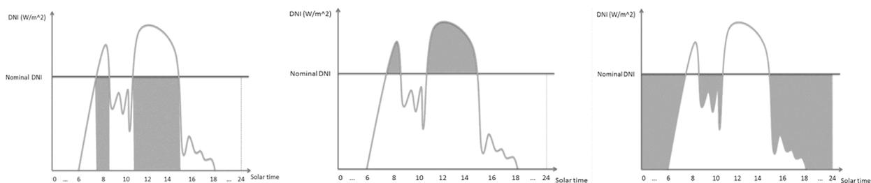
Fig. 1: From left to right: Directly useful radiant energy collected during a generic day (shaded area), excess radiant energy collected during a generic day (shaded area), energy needed to be supplied by the auxiliary systems to ensure an all-day operation in a generic day (shaded area)
