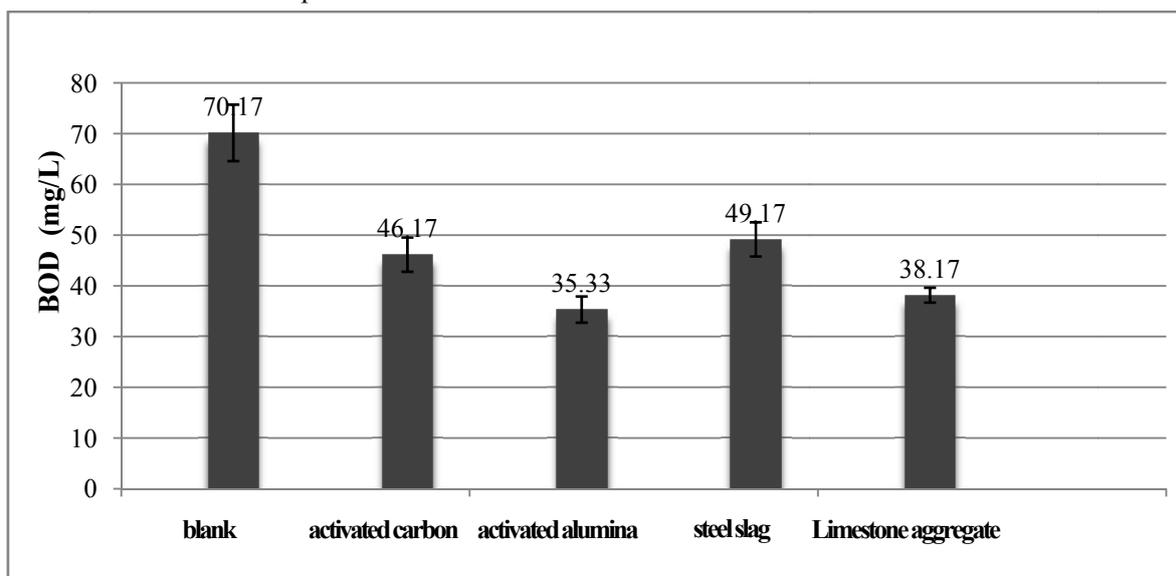
Fig. 2: Effect of Different Adsorbents on BOD Removal
