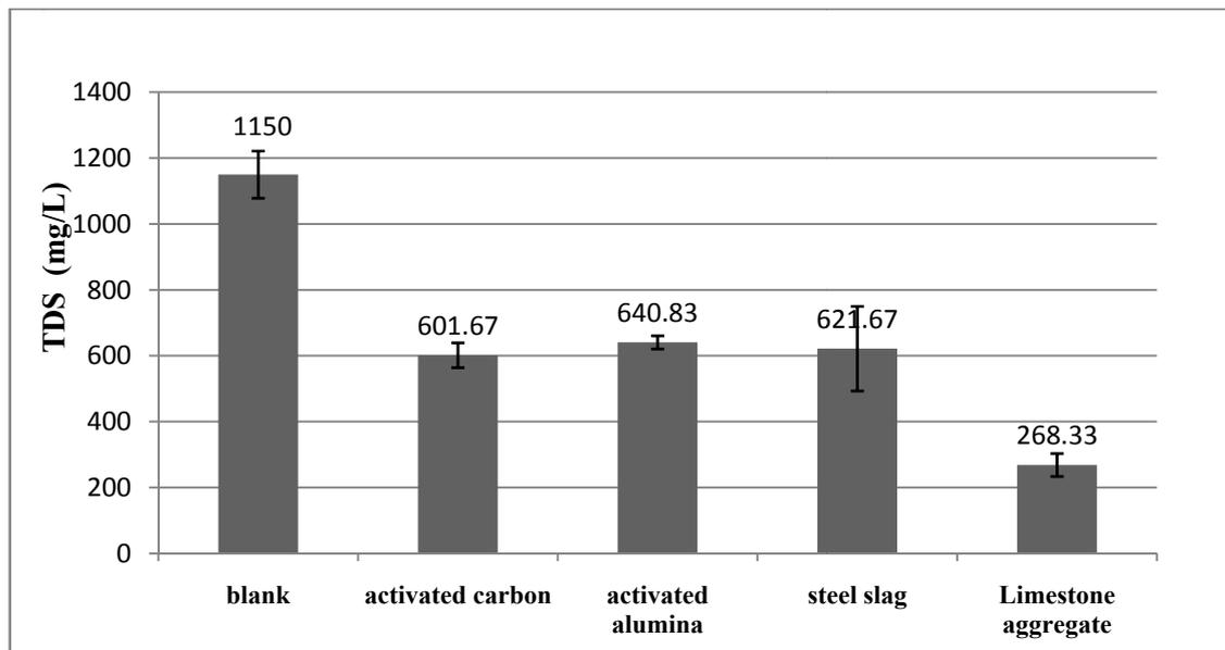
Fig. 1: Effect of Adsorbents on TDS Removal
