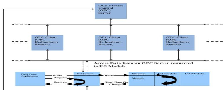
Fig. 3: Continuous Process Control Monitoring Automation System
