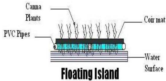
Fig. 1: Schematic Diagram of Floating Island
