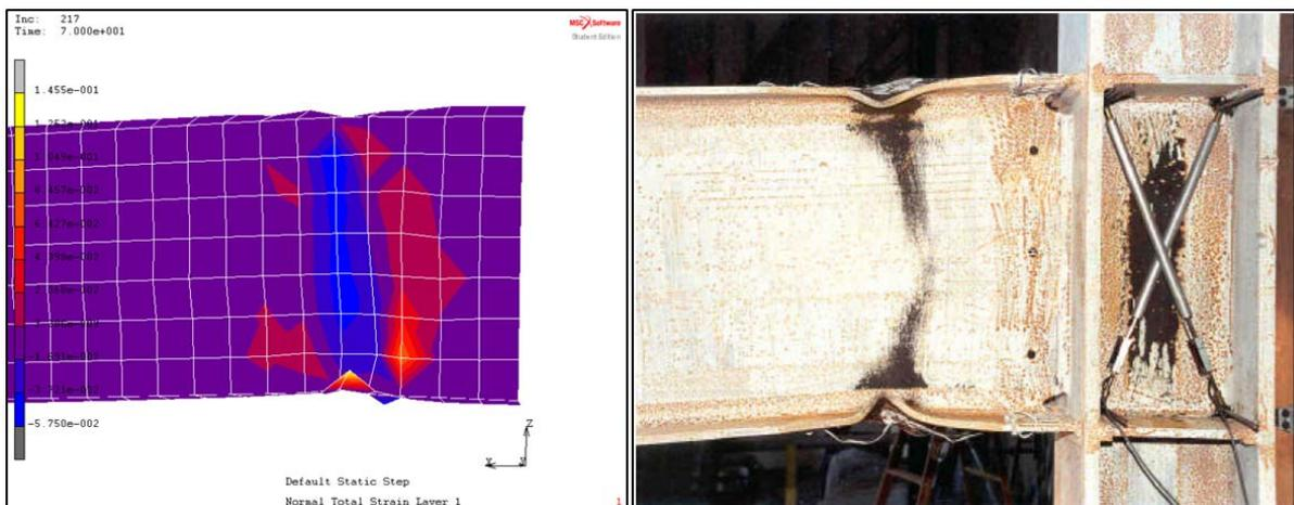
Fig. 6: Comparison of the model vs. the experiment at 5% drift.
