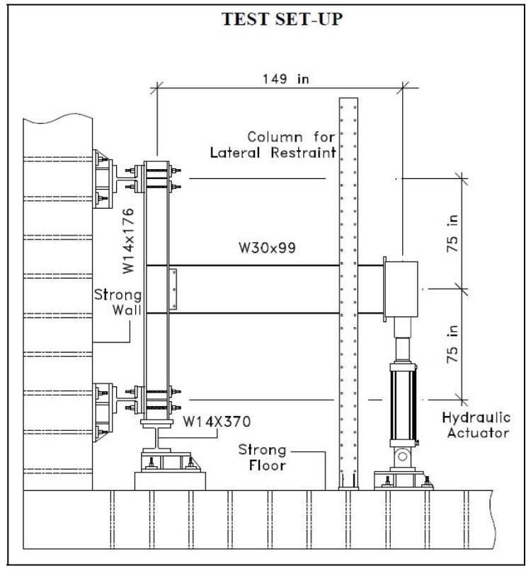
Fig. 1: Test setup in the original experiment in the UCSD Lab from Uang et. al [1] [4].
