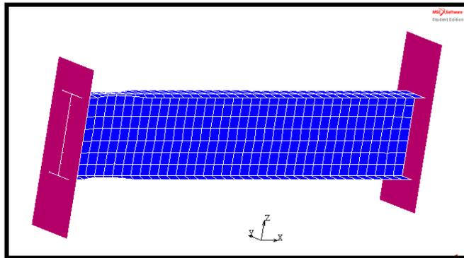
Fig. 4: Added rigid plates used to control the support and loading on sides of the beam.
