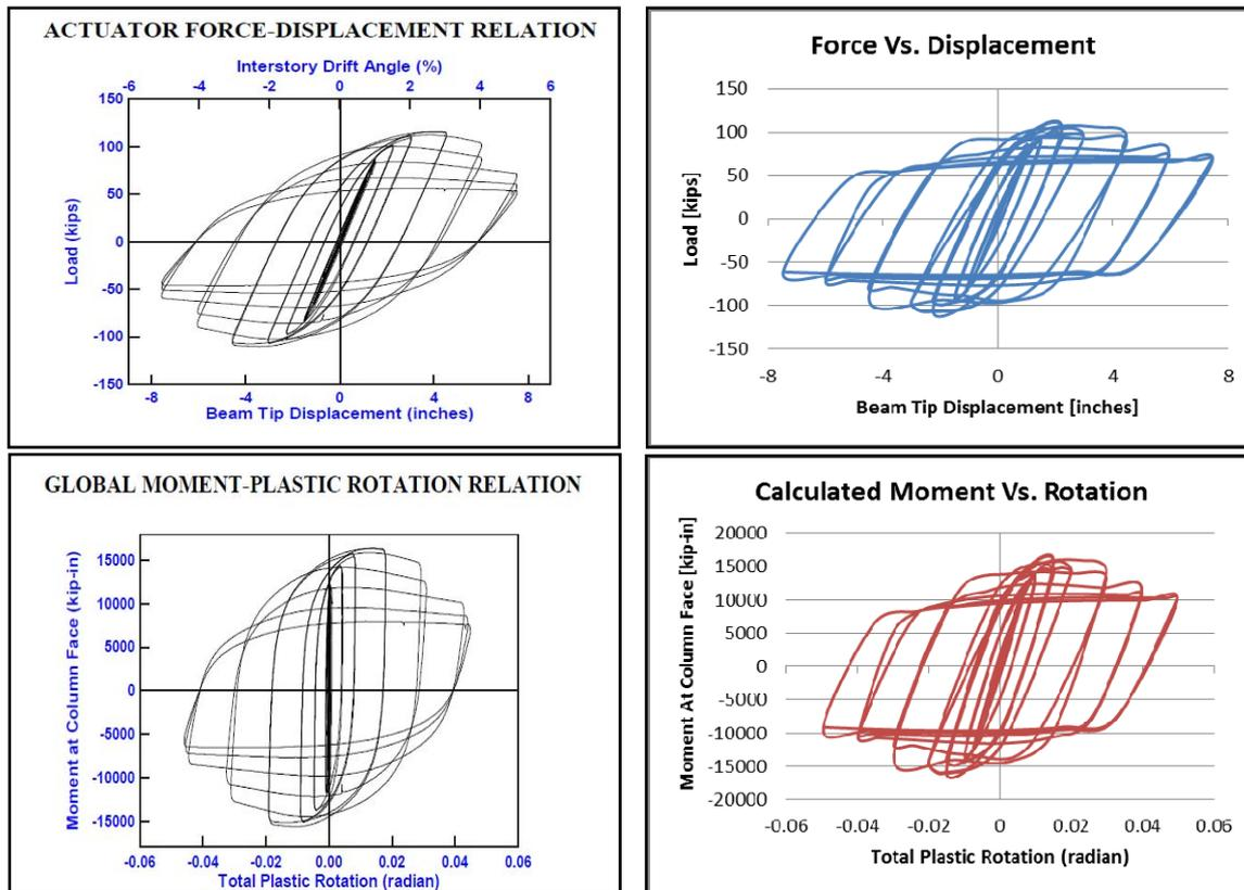
Fig. 7: Comparison between experimental (right) vs. virtual analysis by MSC Marc (left).
