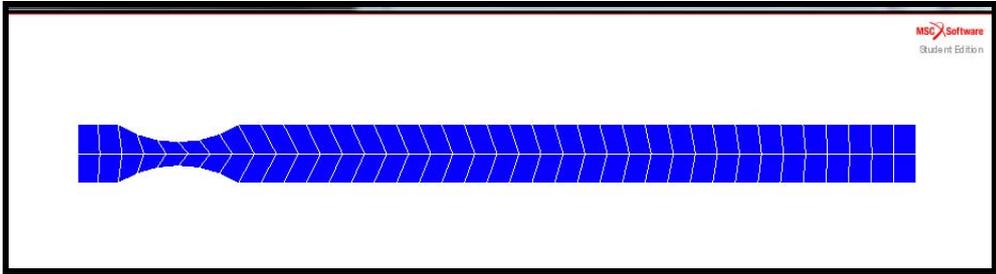
Fig. 3: Steel beam imported and meshed in Patran (top View).
