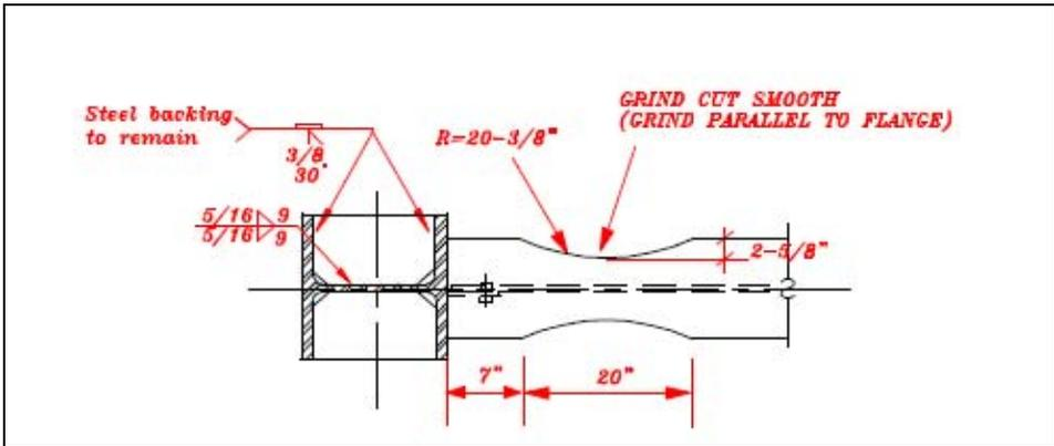
Fig. 2: RBS details at the face of the column from the UCSD Lab report by Uang et. al [1] [4].
