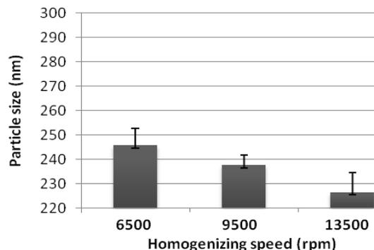
Fig. 4: Effect of homogenizing speed on particle size
