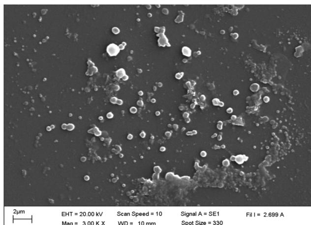
Fig. 6: Electron micrograph of sericin nanoparticle produced from water in silicone emulsion technique
