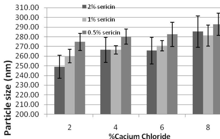
Fig. 2: Sizes of sericin nanoparticles produced with various conditions
