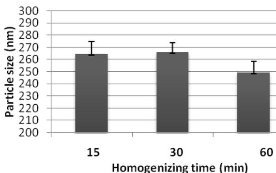
Fig. 5: Size of sericin nanoparticles produced with homogenizing speed 1000 rpm at different of homogenizing times
