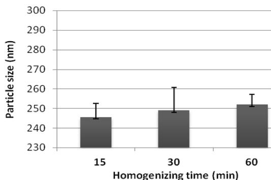
Fig. 3: Effect of homogenizing time on particle size
