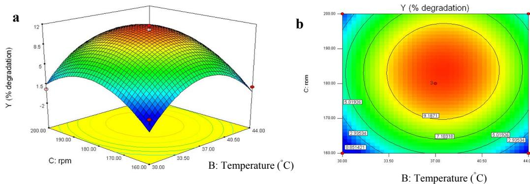
Fig. 3: (a) Response surface plot and (b) its contour plot of the effects of rpm and temperature (°C) and their mutual interactions to determine percentage of PLA degradation by *A. migulanus*.
