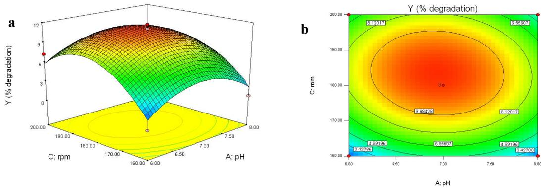
Fig. 2: (a) Response surface plot and (b) its contour plot of the effects of rpm and pH and their mutual interactions to determine percentage of PLA degradation by *A. migulanus*.
