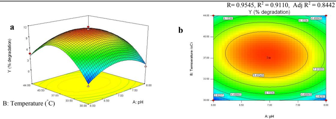
Fig. 1: (a) Response surface plot and (b) its contour plot of the effects of temperature (°C) and pH and their mutual interactions to determine percentage of PLA degradation by *A. migulanus*.
