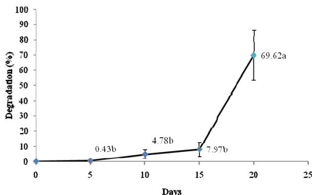
Fig. 4: The percentage of PLA degradation by *A. migulanus* at pH 8,  $40.5^{\circ}\text{C}$  and 194 rpm within 20 days. Values were expressed as means of three replicate analyses  $\pm$ SD.
