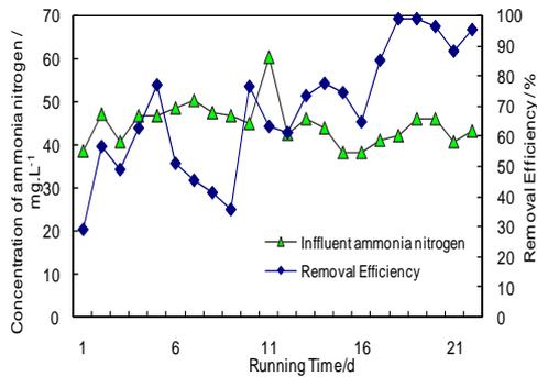
Figure 3. Influent concentration and removal efficiency of ammonia nitrogen in the third and fourth domestication period
