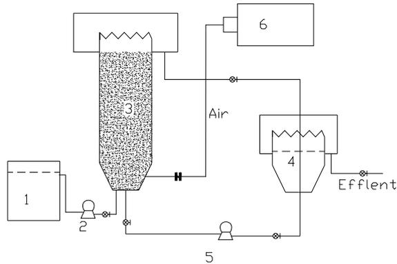
1-Wastewater tank; 2- peristaltic pump; 3- aerobic biological fluid-bed; 4- sedimentation tank; 5- Sludge pump; 6- Gas pump
