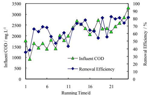
Figure 2. Influent concentration and removal efficiency of COD in the third and fourth domestication period
