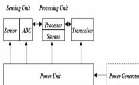
Figure:1 sensor node architecture[2]
