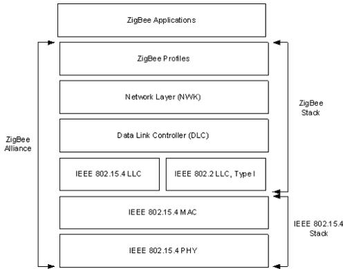
Figure 5: Zigbee protocol stack [6]
