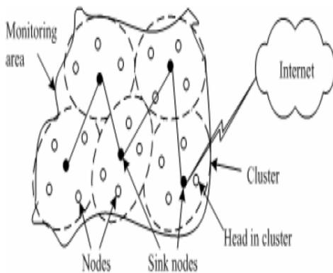
Figure 2: Wireless sensor network architecture [1]
