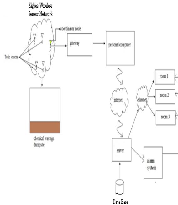
Figure 6: Real time monitoring of chemical wastages by using Zigbee wireless sensor network to control environmental hazards:
