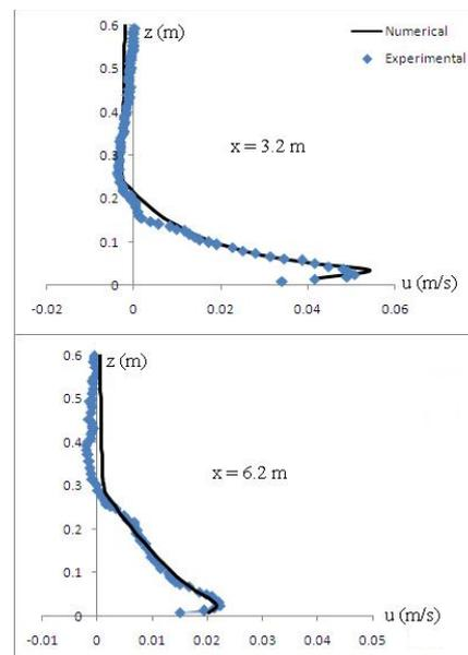
Figure 2. Vertical velocity profiles upstream and downstream of obstacle
