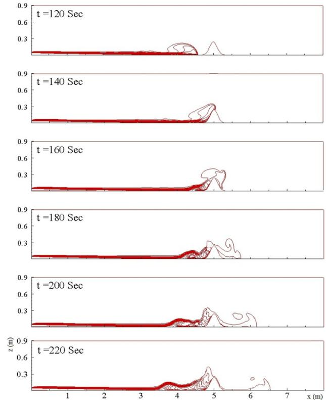
Figure 1. Numerical simulation of turbidity current influenced by obstacle for time steps of 20 s. Lines of equivalent concentration are shown with intervals of 0.1 g/L.
