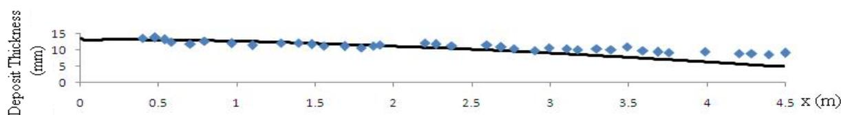
Figure 3. Measured (points) and computed (solid line) deposit thickness upstream of the obstacle
