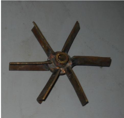
Figure 2. Impeller Used in the Experiments
