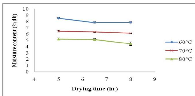
Fig. 1: Moisture content of instant mashed potato after different drying conditions.
