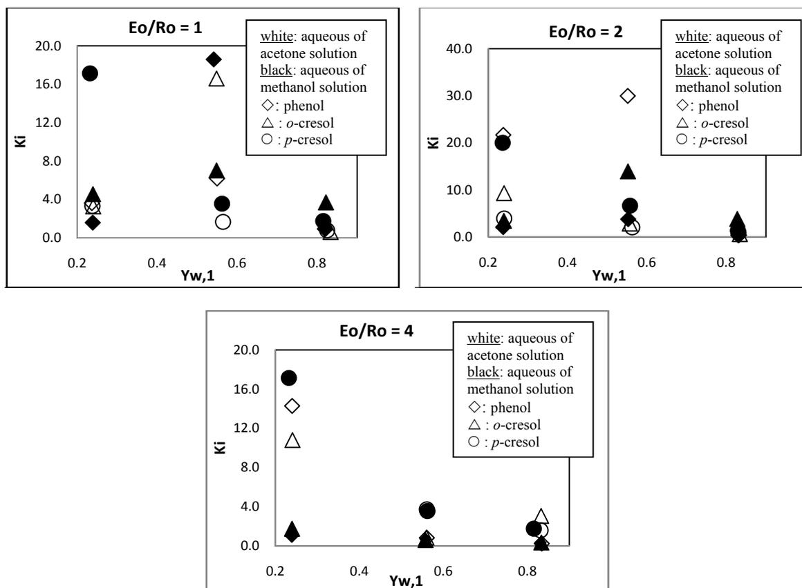
Fig. 1: Effect of mass fraction of water in extract,  $y_w$ , and mass ratio of solvent to feed,  $E_o/R_o$ , on the distribution coefficient,  $K_i$
