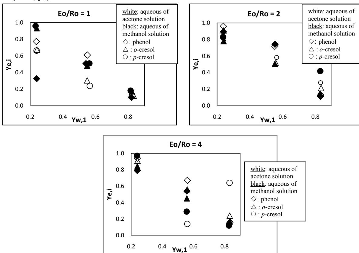
Fig. 2: Effect of mass fraction of water in extract,  $y_w$ , and mass ratio of solvent to feed,  $E_o/R_o$ , on yields,  $y_{e,i}$
