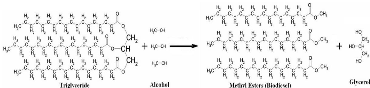
Fig. 1: Alcoholysis process
