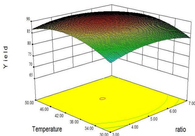
Fig. 2: Effect of methanol ratio and temperature on Yield
