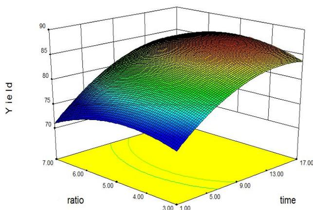
Fig. 3: Effect of methanol ratio and time on Yield
