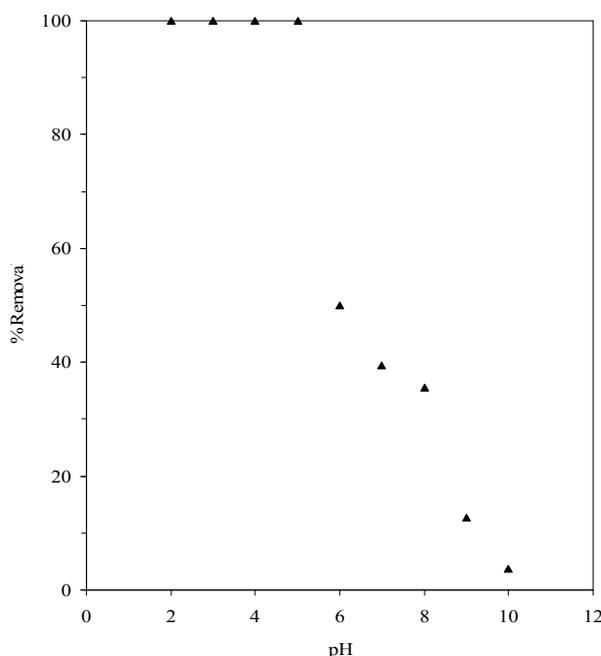
Fig. 1: Effect of pH in the colour removal by MRH from textile wastewater
