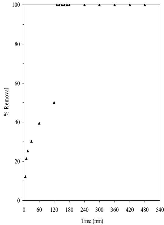
Fig. 2: Effect of contact time in the colour removal by MRH from textile wastewater.
