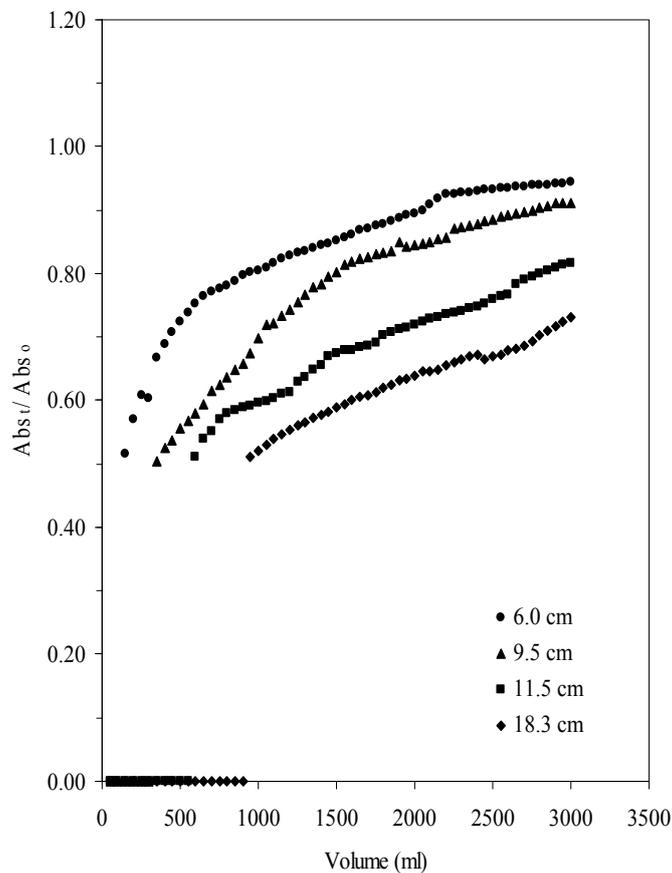
Fig. 3: Breakthrough curves of textile wastewater at different bed depths at a flow rate of 10 mL/min.
