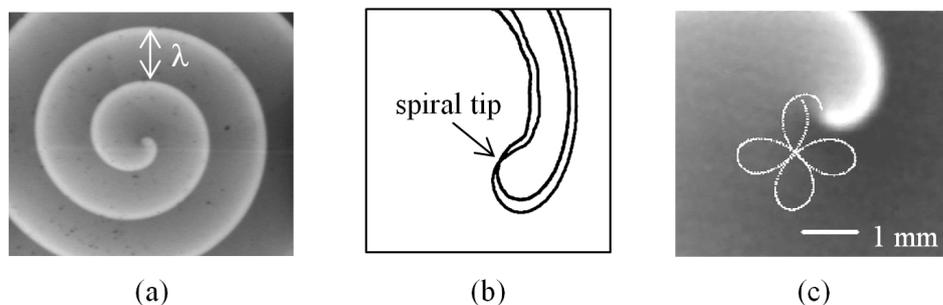
Fig. 2: Analysis of spiral wave dynamics. (a) Image of a spiral wave. Its wavelength  $\lambda$  is the distance between adjacent fronts. (b) The spiral tip is defined as the intersection of contour lines of two consecutive spiral images. (c) The spiral tip trajectory is a temporal set of spiral tip locations. A 4-petal meandering pattern is traced by the spiral tip during 30 min.
