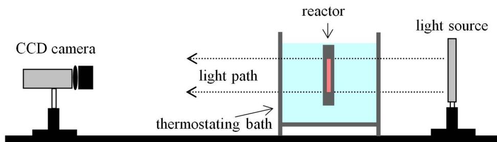
Fig. 1: Experimental setup. A flat reactor containing a thin layer of BZ medium is placed in a thermostating bath to control the temperature. The BZ medium is illuminated by a white light source and observed by a CCD camera.
