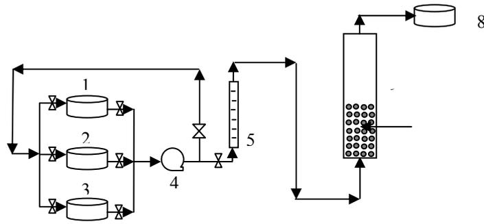
Fig. 1: Experimental system: (1) NaNO<sub>3</sub>, (2) H<sub>2</sub>O, (3) NaOH, (4) Pump, (5) Rotameter, (6) Column, (7) Resin, and (8) effluent.
