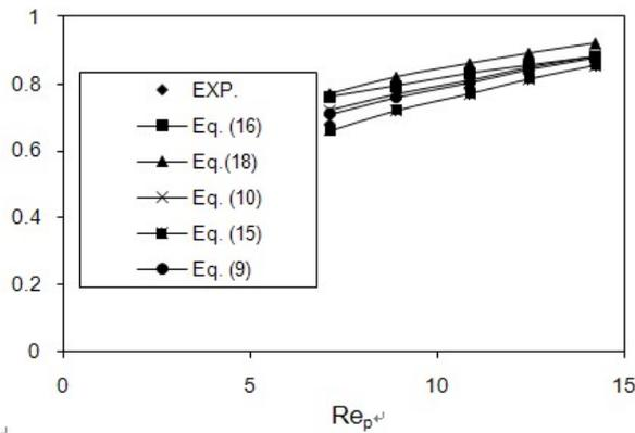
Fig. 4: Comparison of overall voidage estimation models with experimental data
