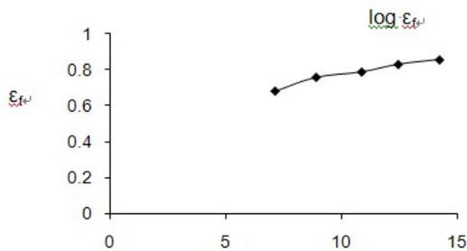
Fig. 2: Effect of  $Re_p$  on fluidized bed voidage ( $\epsilon_f$ )
