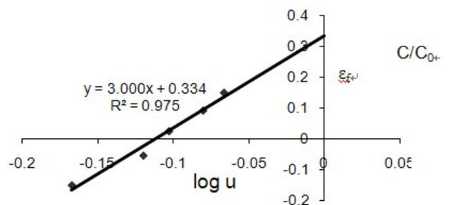
Fig. 3: Richardson-zaki correlation between flow velocity and bed voidage for determination of  $n$  and  $U_t$
