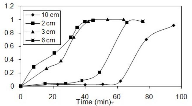
Fig. 5: Breakthrough curves of  $\text{NO}_3$  ions in the fluidized bed at different bed heights  $Z$  and a constant flow rate of 2 L/h
