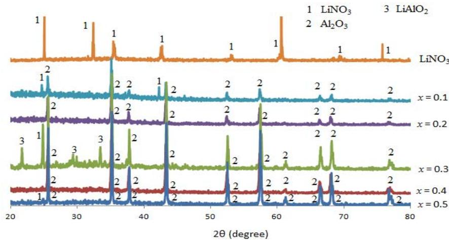
Fig. 1: X-ray diffraction patterns of pure  $\text{LiNO}_3$  and  $(1-x)\text{LiNO}_3-x\text{Al}_2\text{O}_3$  composites.
