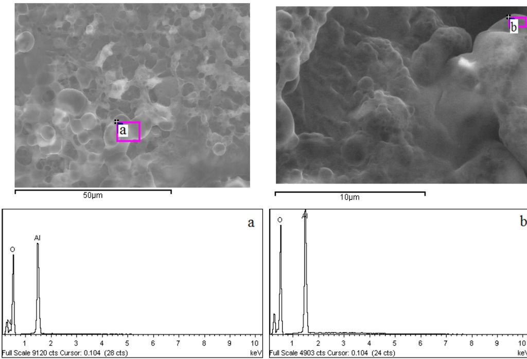
Fig. 4: EDX analysis of the composite sample with  $x = 0.3$  at different points.
