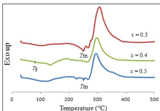
Fig. 2: DSC curves for  $(1-x)\text{LiNO}_3-x\text{Al}_2\text{O}_3$  composites.
