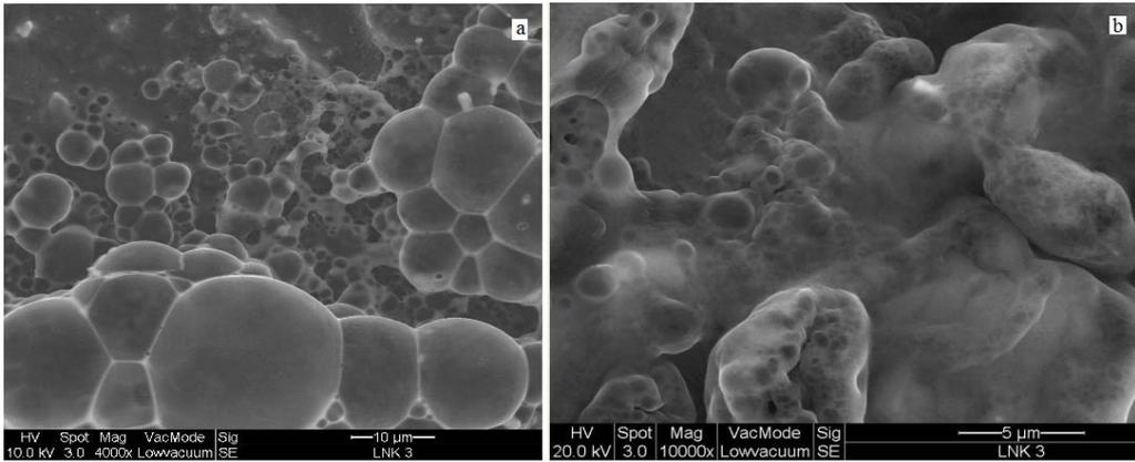
Fig. 3: SEM images of the composite sample with  $x = 0.3$  (a) surface morphology and (b) cross section.
