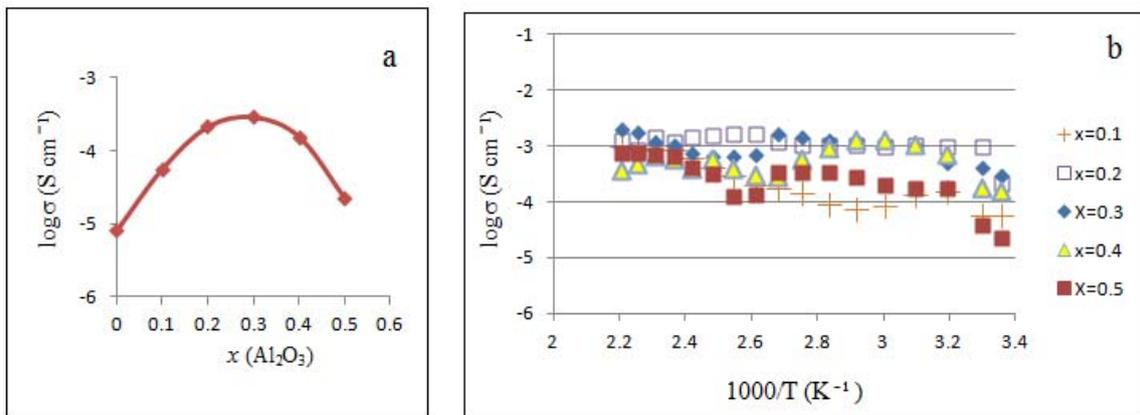
Fig. 5: Arrhenius plots of conductivity at room temperature (a) and  $\sigma(x)$  dependences (b) for  $(1-x)\text{LiNO}_3-x\text{Al}_2\text{O}_3$  composites.
