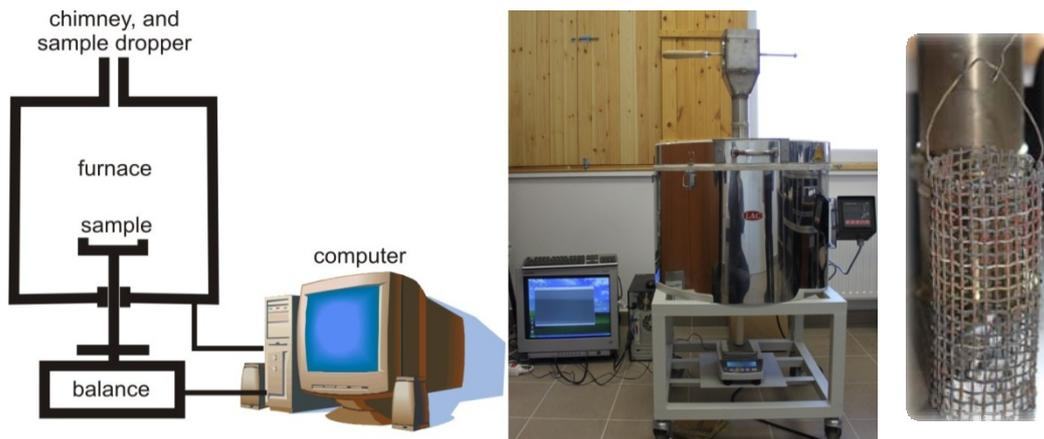
Fig. 4: The experimental assembly, the oven and the sample holding basket
