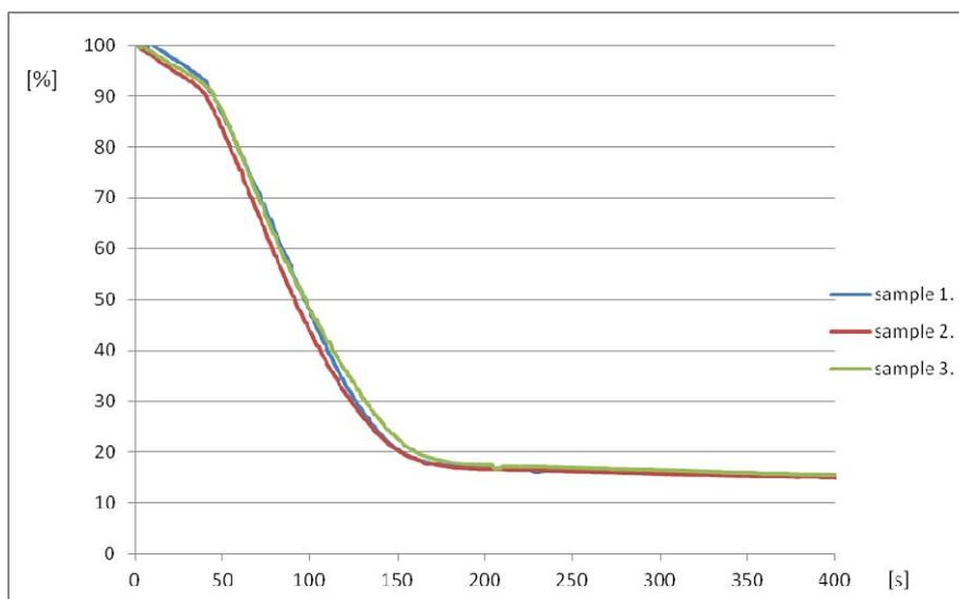
Fig. 5: Combustion dynamics image of repeated measurements overlapping and showing the balanced state of combustion
