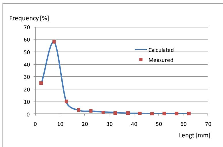
Fig. 1: Size composition of chopped green maize forage (adjusted length 5 mm)
