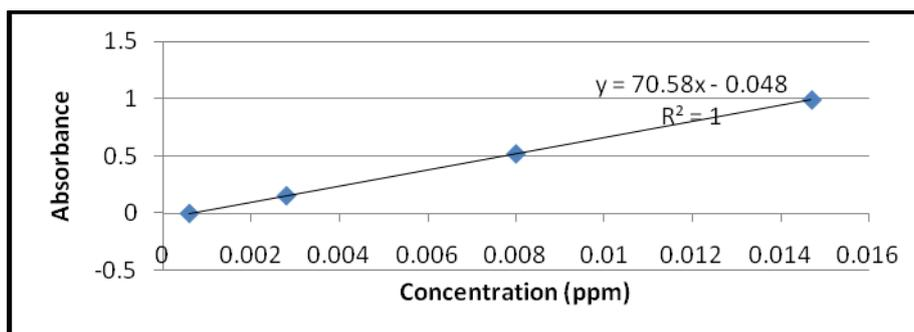
Fig 2: Graph of Chromium Standard Calibration [Concentration (ppm) vs Absorbance]
