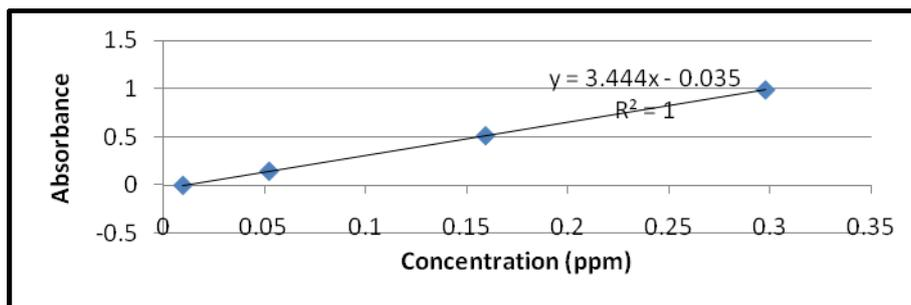
Fig 1: Graph of Cadmium Standard Calibration [Concentration (ppm) vs Absorbance]
