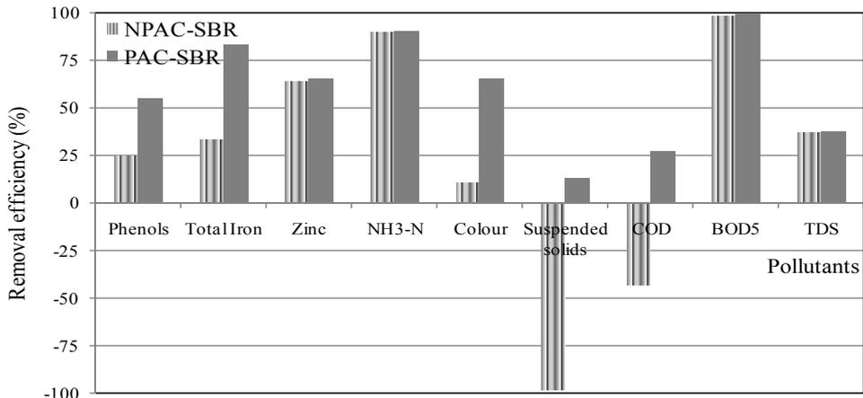
Fig. 1: Removal efficiencies of risky pollutants inside NPAC- and PAC-SBRs
