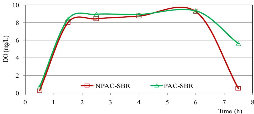
Fig. 2: A sample of DO variation inside the reactors
