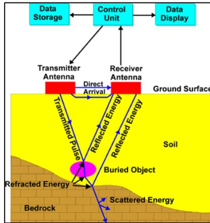
Fig. 1: EM wave propagation depends on dielectric and conductivity properties of material [5].
