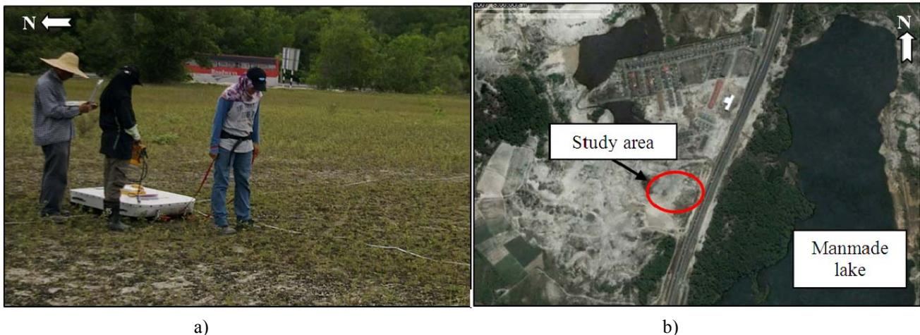
Fig. 2: Ground penetrating radar. a) 100 MHz shielded antenna used in the study, b) study area across the sandy soil.
