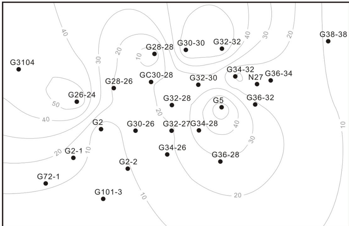
Fig.2 Distribution of Bottom fluid pressure in block G5
