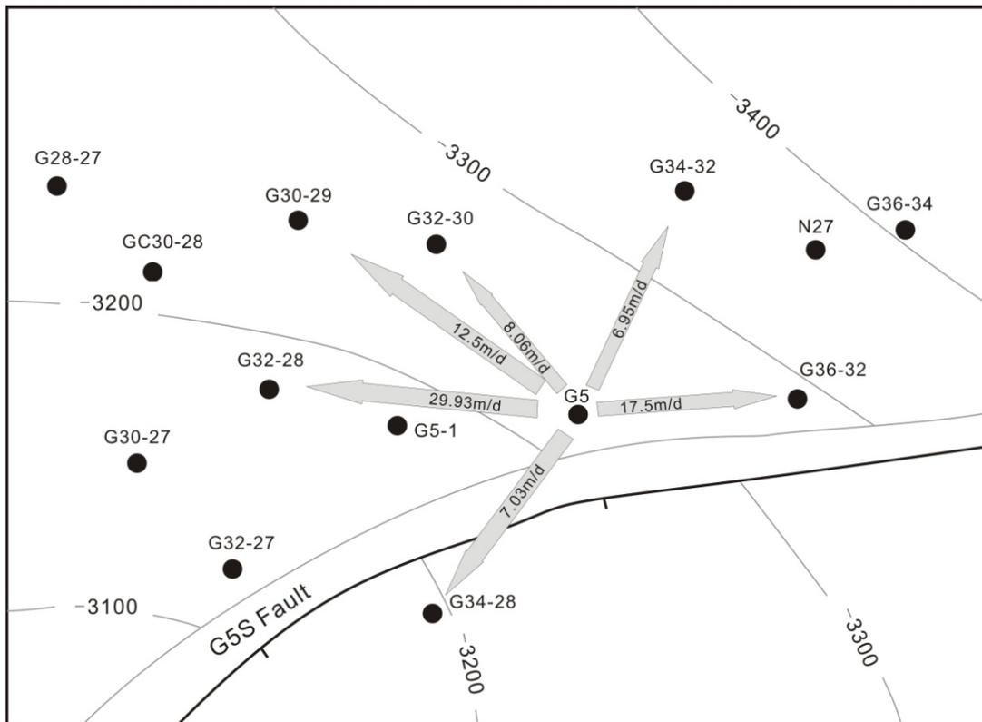
Fig.3 Expanded direction and velocity of water flooding in G5 well groups
