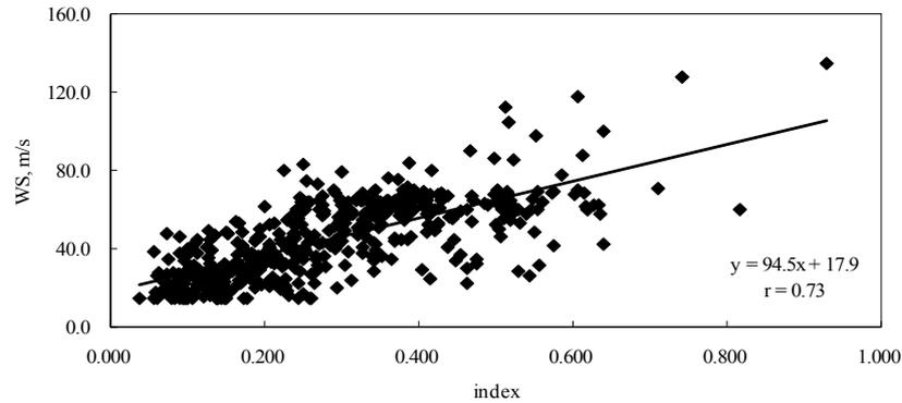
Fig. 2 The correlation distribution between wind speed (WS) and index of typhoons from TD to severe stage
