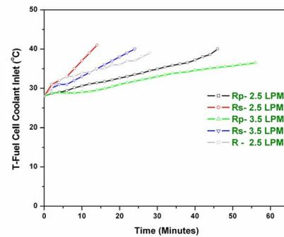
Fig.4: Primary coolant inlet temperature profile
