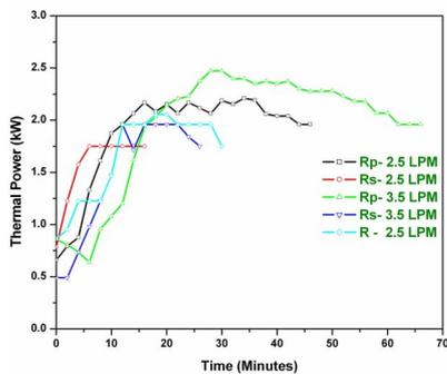
Fig.3: Heat removal from fuel cell profile
