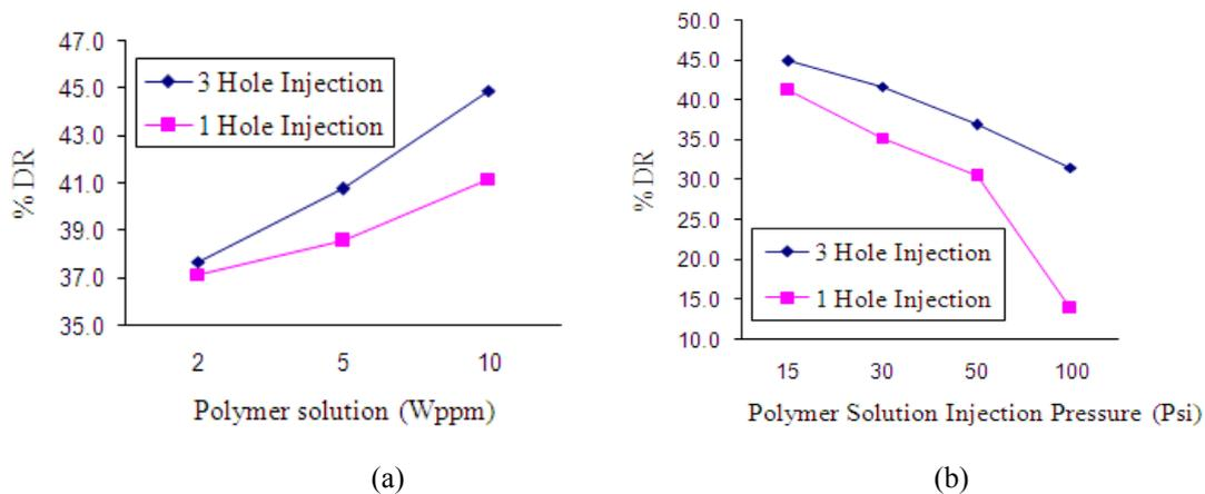
Fig. 1: (a) Variation of % DR versus concentration of water soluble polymer solution in pipeline, (b) variation of %DR versus pressure (psi) of polymer injection systems
