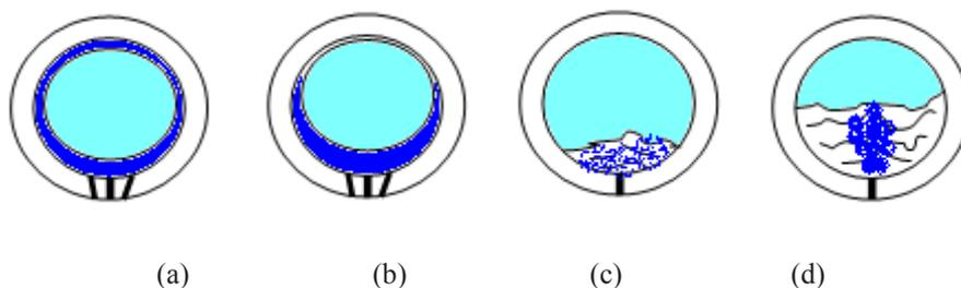
Fig. 2: Polymer film distribution in pipeline (a) 3 hole nozzle at low pressure, (b) 3 hole nozzle at high pressure, (c) single hole nozzle at low pressure, (d) single hole nozzle at high pressure
