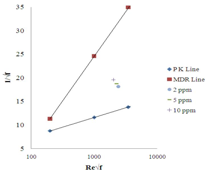
Fig. 3: PK plot for drag reduction asymptote of 10 wppm at 15 psi of PAM (MW  $4 \times 10^6$  g/mol)
