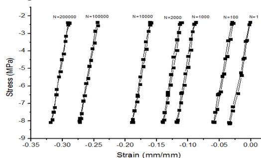
Fig. 1: Stress strain hysteresis for bovine femoral ball.
