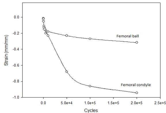
Fig. 3: Maximum strain as a function of numbers of cycles in two different anatomic parts.
