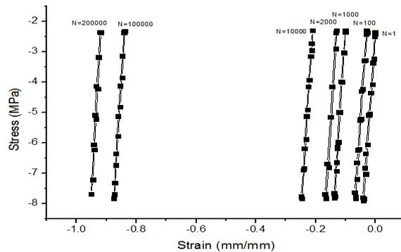
Fig. 2: Stress strain hysteresis for bovine femoral condyle.
