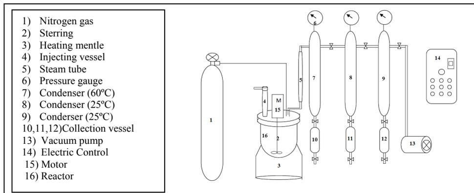
Fig.1: Schematic layout of Pyrolysis system
